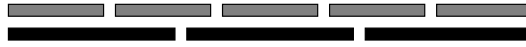
Figure 27: Vernier. Rodlike tiles differing in length form an assembly that grows until the ends exactly match.
